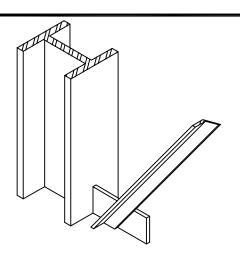
FOR COMPLEX CLUSTERED IRREGULAR SHAPED PENETRATIONS REQUIRING THE USE OF HYDROSEAL 1K, IT WILL BE NECESSARY TO ENCLOSE THE PENETRATIONS IN CONCRETE CURBS.
