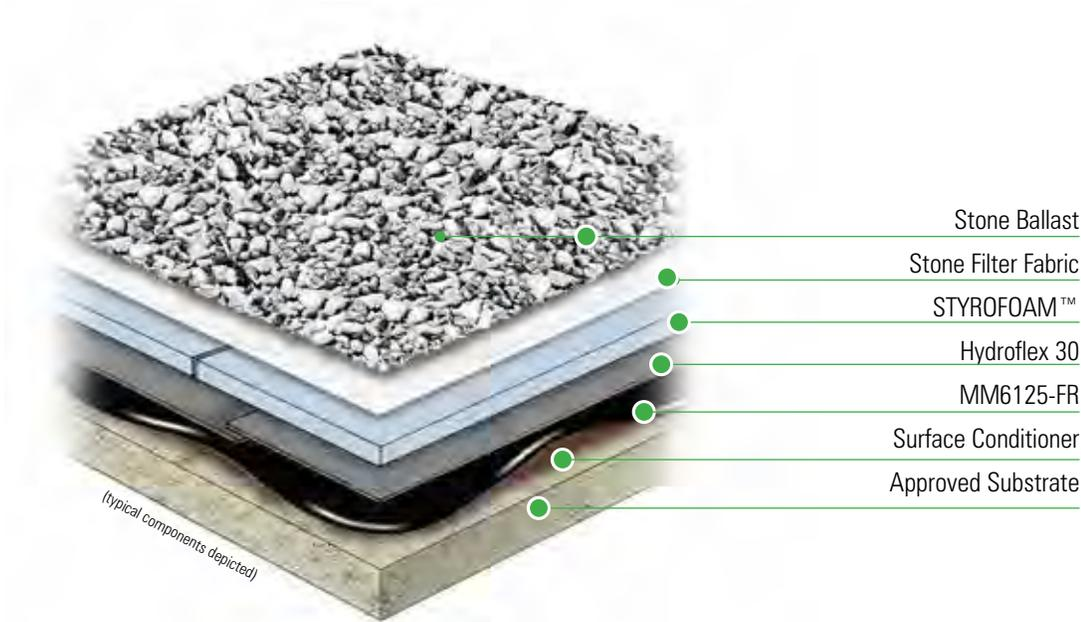
The original and still very practical protected membrane roof (PMR) assembly utilizes crushed or washed stone as the ballasting material over the STYROFOAM™ insulation. Stone provides the weight to keep the insulation materials in place over the membrane.
