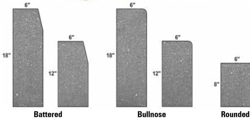
RockCurb precast concrete curbing units can be used to create landscape areas with intensive or extensive assemblies. RockCurb is hydraulically pressed concrete with a minimum strength of 8,500 psf. It comes in eight colors that complement the architectural pavers in the Ultimate Assembly®.
