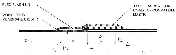
BUILT UP MEMBRANE (ASPHALT OR COAL TAR)
