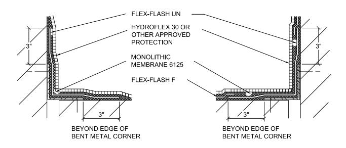
NOTE: FLEX-FLASH F MAY BE USED AT ALL CONCRETE-TO-CONCRETE AND CONCRETE-TO-CONCRETE BLOCK TRANSITIONS. FLEX-FLASH UN MUST BE USED AT ALL OTHER TRANSITIONS.
