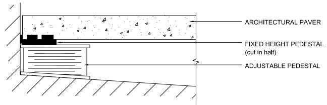
NOTE: AT TYPICAL TERMINATION POINTS, THE ADJUSTABLE PEDESTALS ARE PLACED SUCH THAT 1/2 OF A FIXED HEIGHT PED. MAY BE BUTTED UP TO THE STRUCTURE (curb, wall, etc.).
