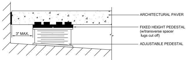
NOTE: IF NECESSARY, THE PAVER MAY BE CANTILEVERED OUT PAST THE LAST ROW OF SUPPORTS. THE CANTILEVER SHOULD NOT EXCEED 3" W/O ADDITIONAL SUPPORT. PROPER EXPANSION/BUFFER MATERIAL SHOULD BE PLACED BETWEEN PAVER AND FLASHING.
