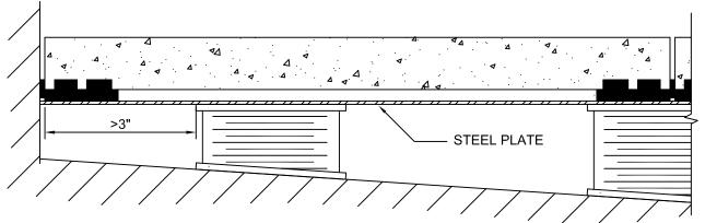
NOTE: WHEN THE LAST PAVER NEEDS TO CANTILEVER > 3", A STEEL PLATE, 5"  $\times$  26"  $\times$  3/8", SHOULD BE LAID TO BRIDGE BETWEEN THE LAST 2 ADJUST. PED. FIXED HEIGHT PEDS. ARE THEN PLACED ON TOP OF THE STEEL PLATE TO SUPPORT AND SPACE THE PAVERS. THE HEIGHT OF THE LAST 2 ROWS OF ADJUST. PEDS. NEEDS TO BE LOWERED, BY THE THICKNESS OF THE STEEL PLATE.
