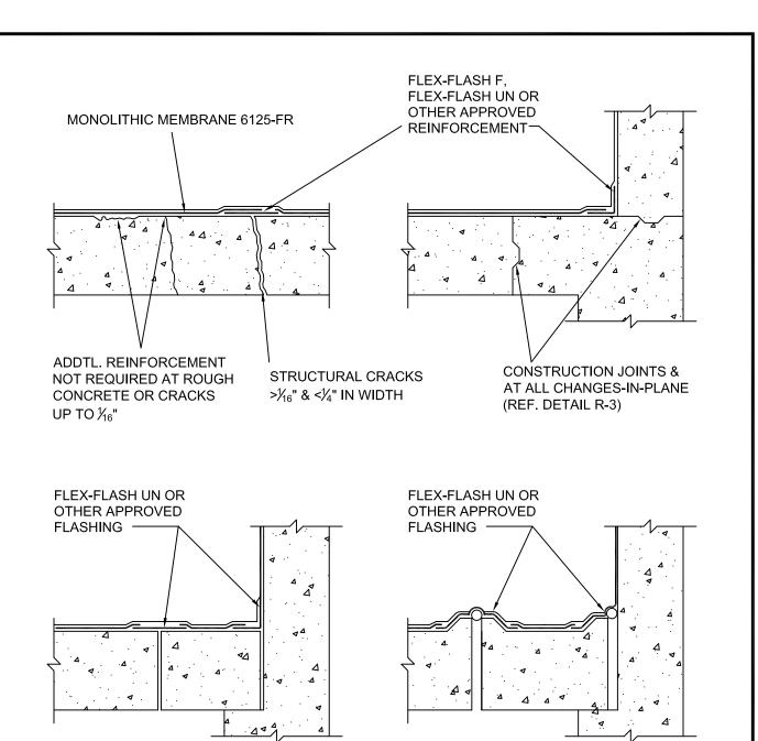
EXPANSION JOINTS UP TO 1" IN WIDTH AND MAX. 25% MOVEMENT ACCOMMODATION FACTOR (REF. DETAIL R-6A)
